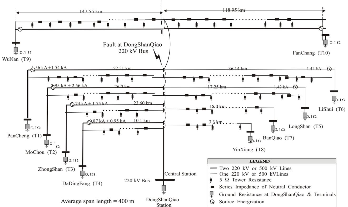
Fig. 10 Circuit Model of the 220 kV Network Used to Determine the Fault Current Distribution
