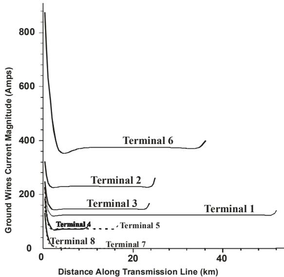
Fig. 11 Computed Fault Current in the Transmission Line Overhead Ground Wires (only one line for each terminal is represented. The currents in the other lines are about the same).
