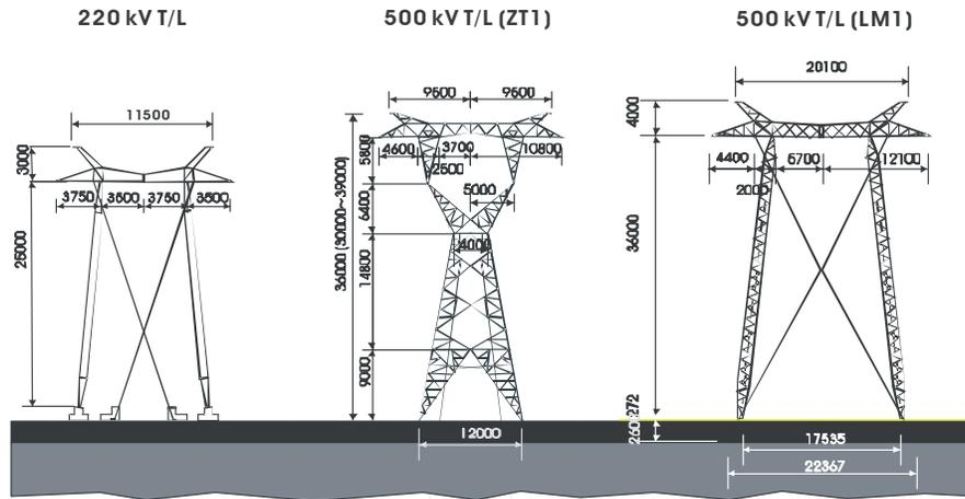
Fig. 9 Cross-Sections of the 500 kV and 220 kV transmission lines
