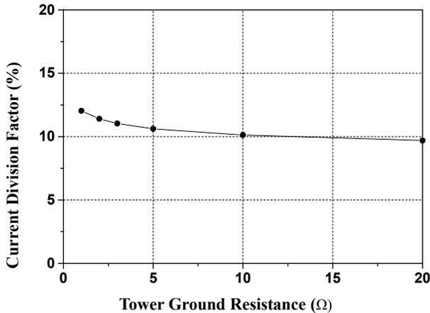
Fig. 7 Current division factor for different tower ground resistances
