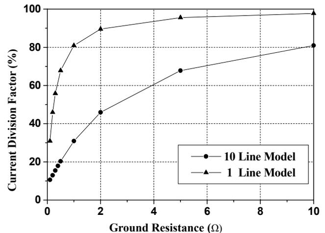
Fig. 5 Current Division Factor for Different Substation Ground Resistances: one line model and ten line model
