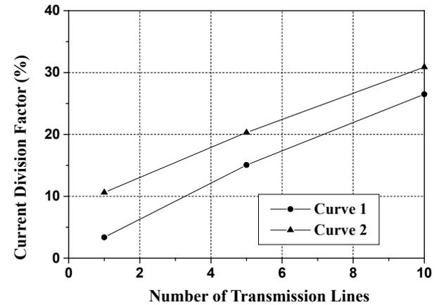
Fig. 3 Current Division Factor with Various Number of Transmission Lines (Substation grounding grid resistance is  $0.1 \Omega$ )
