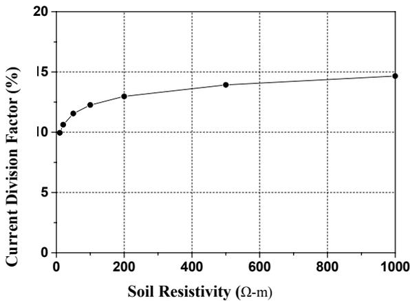
Fig. 6 Current Division Factor for Different Soil Resistivity
