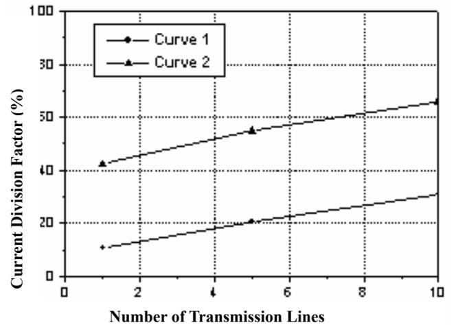
Fig. 8 Current Division Factor for Different Type of Shield Wires
