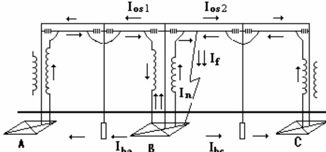
Fig. 1 Distribution of fault current at a station
