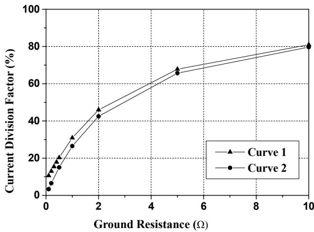
Fig. 4 Current Division Factor with Different Substation Ground Resistances
