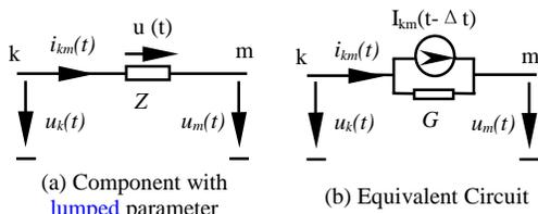
Fig.2. Calculation circuit of Bergeron Method
