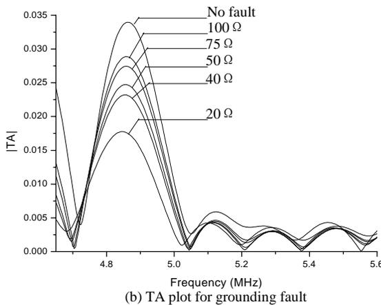
Fig.4. DA and TA of different fault intensities in disc #18
