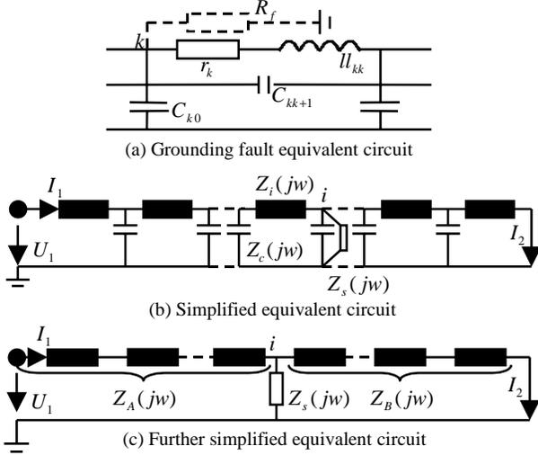
Fig.3. Simplified Circuit
