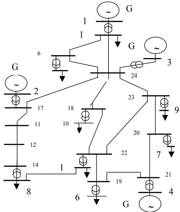
Figure 2 Practical 24-bus EHV equivalent system
