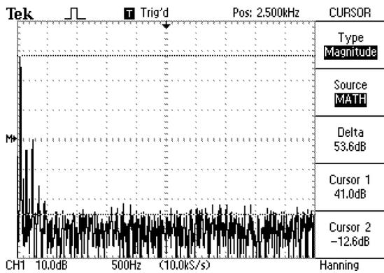
Fig. 11: Output phase voltage frequency spectrum for a 5-level,  $N=5$ ,  $m_a=1.2$ ,  $f_{sp}=20$  kHz.
