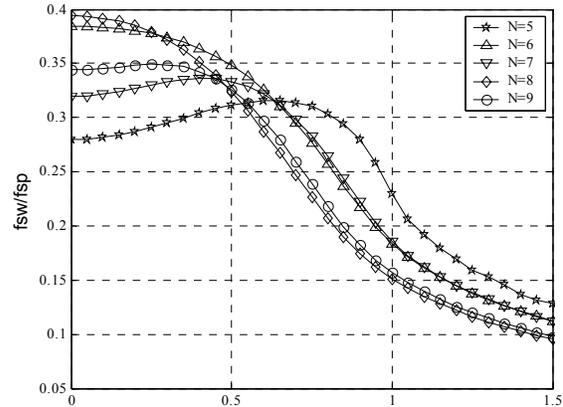
Fig. 10: Predicted  $f_{sw}/f_{sp}$  versus  $m_a$ : 5-level,  $N=6$ ,  $f_{sp}=20$  kHz.
