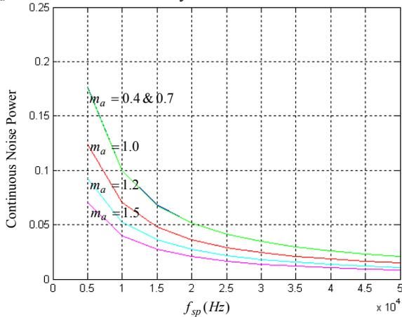
Fig. 9: Predicted discrete noise power versus  $f_{sp}$  for 3-level WRPWM scheme with  $N = 4$ .
