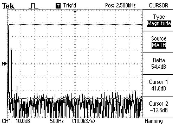
Fig. 12: Output phase voltage frequency spectra for a 5-level WRPWM schemes:  $N=6$ ,  $m_a=1.2$ ,  $f_{sp}=20$  kHz.
