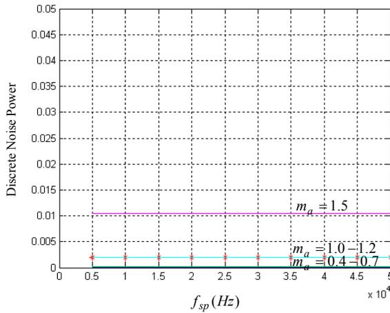
Fig. 8: Predicted discrete noise power versus  $f_{sp}$  for 3-level WRPWM scheme with  $N = 4$ .
