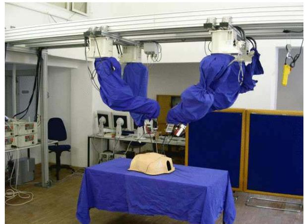
**Figure 2. System setup: Four ceiling mounted robots with three instruments and an endoscopic stereo camera attached. Size of the system (including gantry) is approx. 2.5m x 5.5m x 1.5m.**
