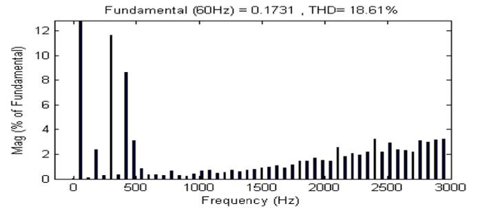
Fig. 9. Harmonic spectrum of the leakage current for a fault in the 10<sup>th</sup> tower and capacitance  $C_3$ .
