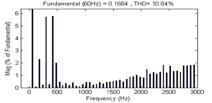
Fig. 7. Harmonic spectrum of the leakage current for a fault in the 1<sup>st</sup> tower and capacitance  $C_3$ .
