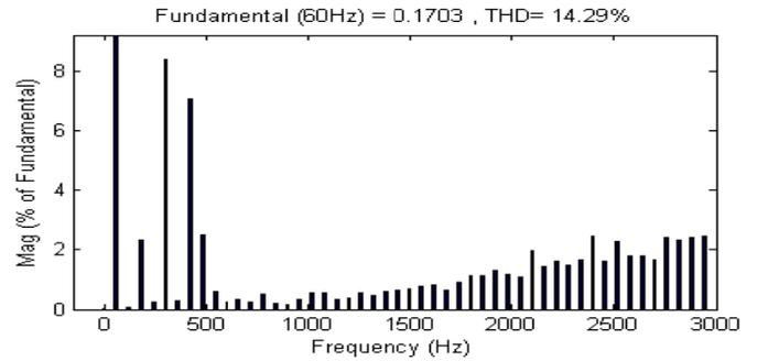
Fig. 8. Harmonic spectrum of the leakage current for a fault in the 5<sup>th</sup> tower and capacitance  $C_3$ .
