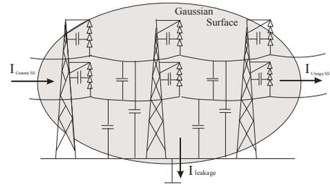
Fig. 5. Gaussian closed surface for the stretch of a TL.
