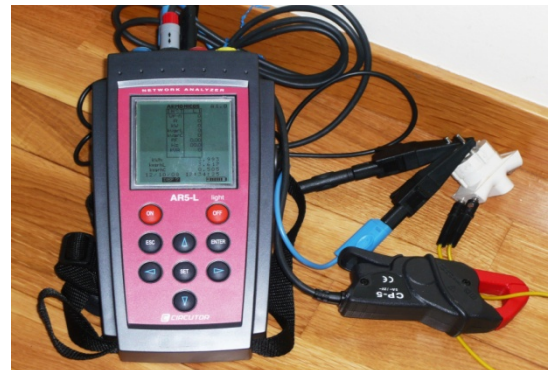
Fig. 3. Supply network analyzer AR5L of CIRCUTOR.
