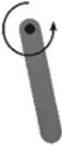
Figure 7. Pendulum system, which consists of a pole and the goal of the task is to swing the pole up so it stays upright.
