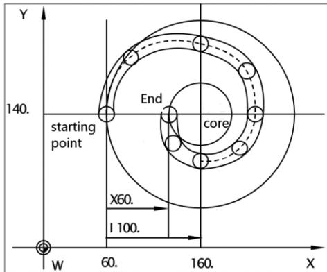
Figure 6. Vortex/conic insertion.
