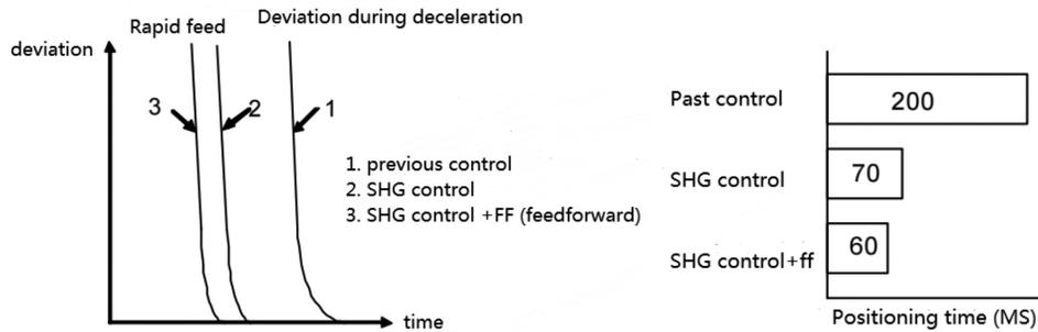
Figure 11. Comparison of positioning time and dosage.
