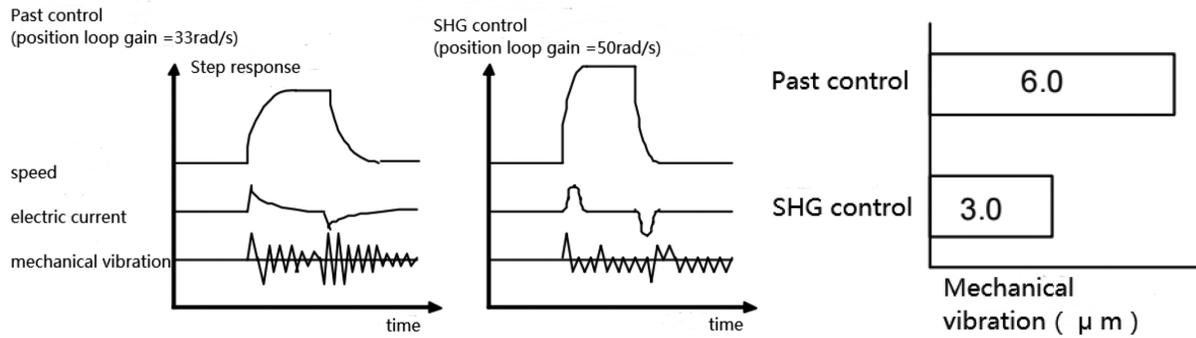
Figure 9. SHG control and mechanical vibration amount comparison.
