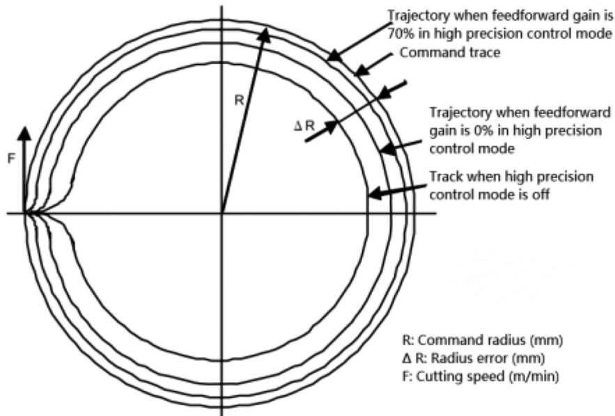
Figure 1. The effect of G 0 2 and G 0 3 interpolation in the circular arc.
