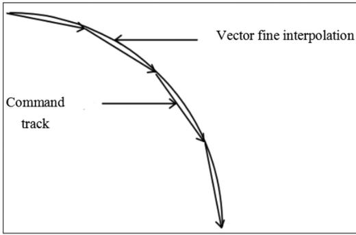
Figure 4. High-precision vector interpolation.
