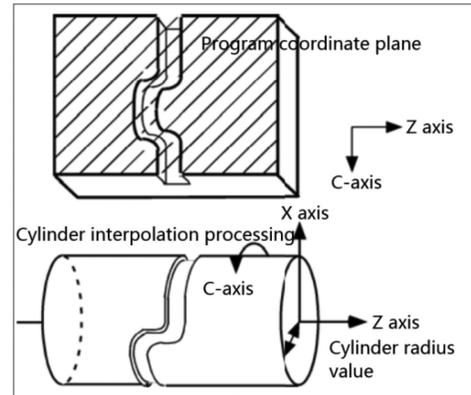
Figure 7. Cylinder insertion.
