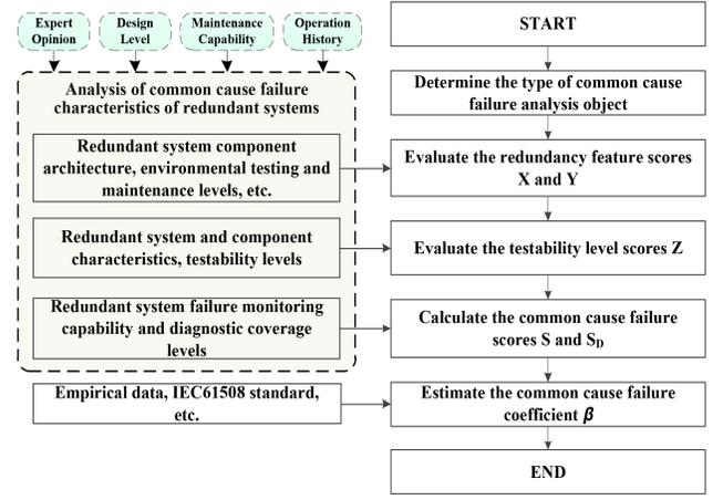
Figure 2. The process of estimation  $\beta$  value.
