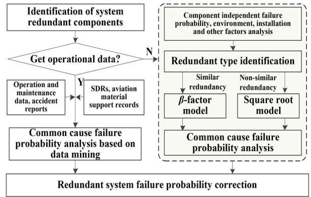
Figure 1. System failure probability correction.
