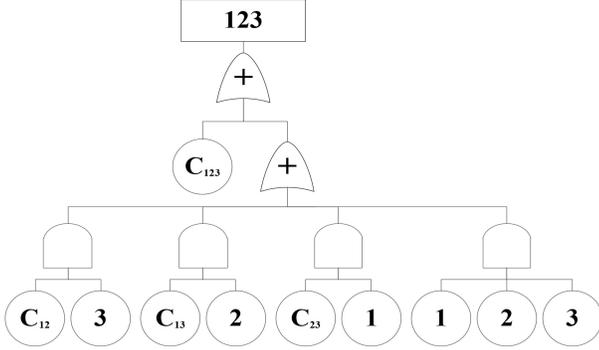
Figure 5. Fault tree of tri-redundancy TRU.
