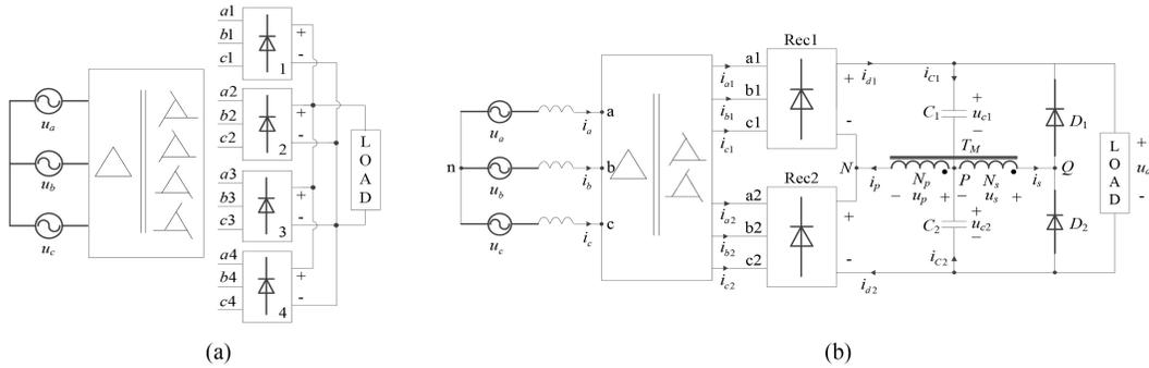
Figure 4. Circuits of the ordinary and new TRU: (a) the ordinary TRU and (b) the new TRU.
