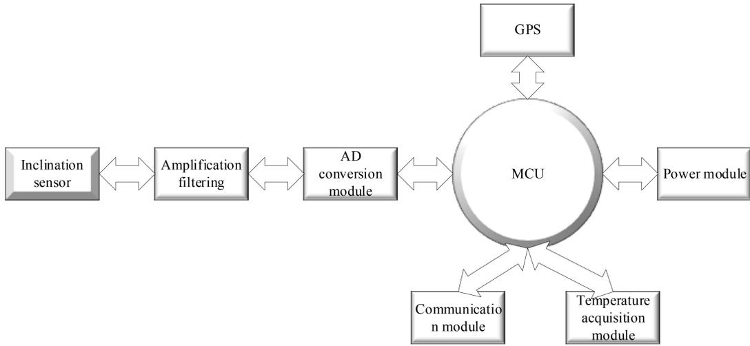
Figure 1. Overall hardware design of arc remote monitoring terminal.
