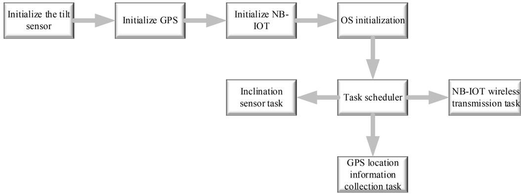
Figure 3. Overall design of remote monitoring terminal software.
