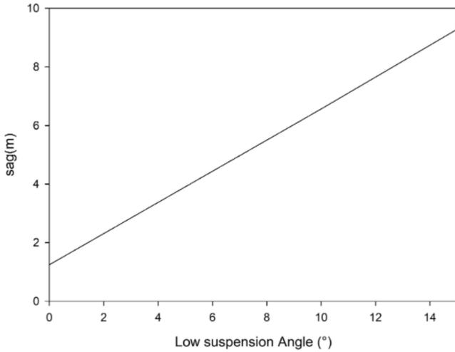
Figure 8. The relationship between suspension point and maximum sag when the spacing is 120 m and the height difference of suspension point is 3 m.
