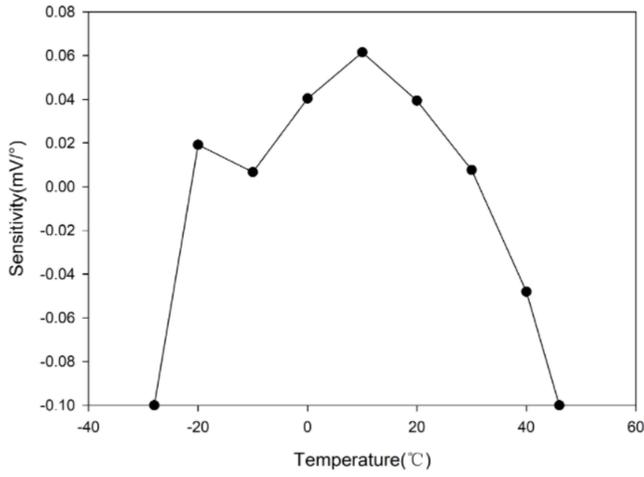
Figure 11. Relation between sensitivity compensation and temperature.
