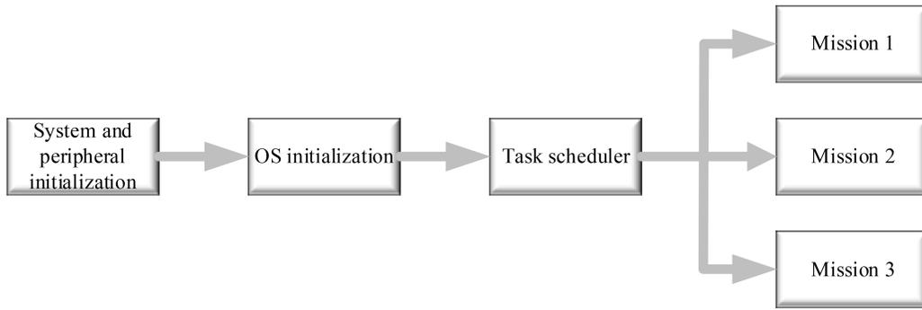
Figure 2. FreeRTOS real-time operating system working principle.
