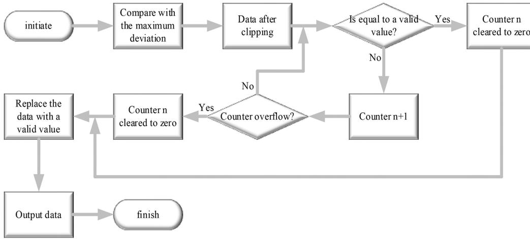
Figure 5. Digital filter design flow.
