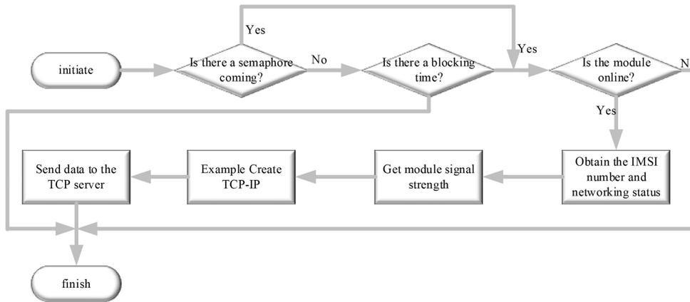
Figure 6. BC28 communication program design flow.
