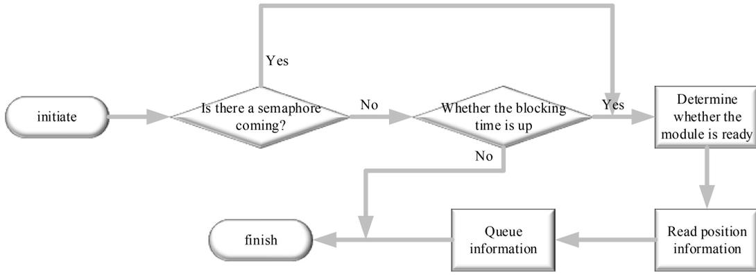
Figure 7. Software design flow of GPS module.
