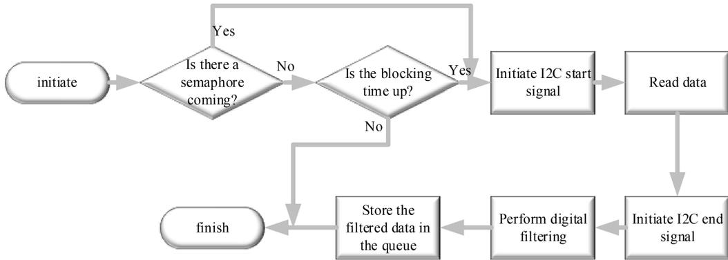
Figure 4. Data acquisition and processing task design of inclination sensor.
