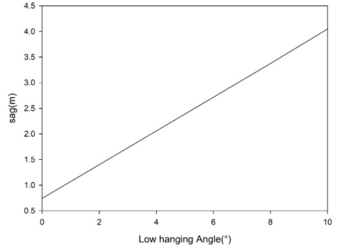
Figure 9. The relationship between suspension point and maximum sag when the spacing is 75 m and the height difference of suspension point is 3 m.
